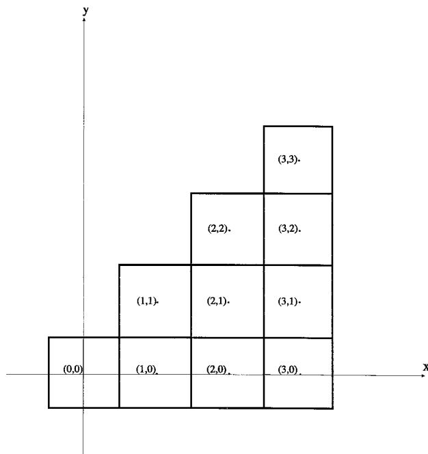
Fig. 4. CCD pixel locations in which signal power is computed for a single input SLM pixel, to show roll-off of the point-spread function.
